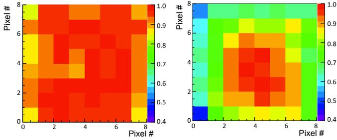
Figure 3: (Left) Example of MAPMT efficiency map normalized to the maximum pixel efficiency. Data show an almost flat behavior at values close to 1 except for the edge pixels. (Right) Example of MAPMT gain map normalized to the maximum pixel gain. The visible 1:2 variation is expected for this type of sensors and can be compensated by the electronics.
