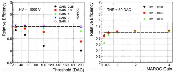
Figure 4: Relative SPE detection efficiency as a function of the working parameters: bias voltage, MAROC preamplification gain and discriminator threshold. The plots show the dependence on two parameters while keeping fixed the third: bias voltage (left) or threshold (right). Data are normalized to the reference point at HV=-1000 V, gain=1 and threshold=+50 DAC. Values greater than 1 are likely due to the cross-talk contribution.
