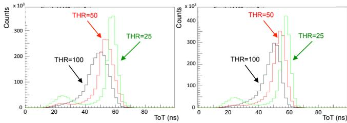
Figure 6: ToT distributions of the RICH channels at three typical values of threshold (25, 50 and 100 DAC) without (left) and with (right) gain equalization. The saturated SPE signals generally yield ToT duration greater than 40 ns. When lowering the threshold also weaker cross-talk signals are recorded with ToT duration around 25 ns.
