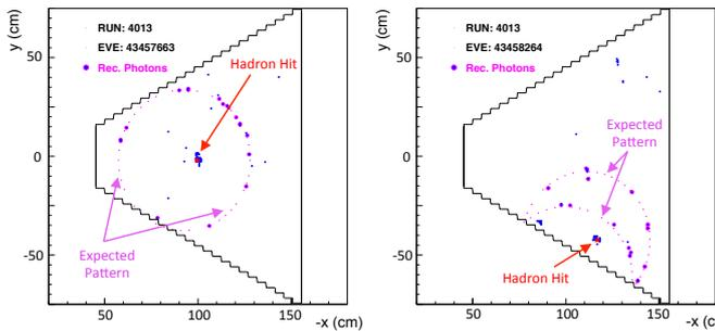
Figure 7: Examples of RICH reconstructed events: direct (left) and partial reflected (right). Big dots indicate the reconstructed photon hits. The arrows indicate the hadron impact point (red star) and the expected photon pattern (small magenta points).
