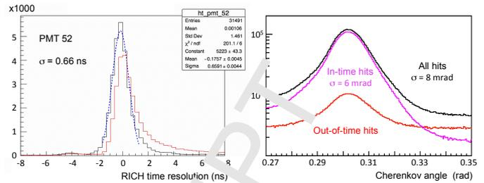
Figure 8: (Left) Typical time resolution before (red) and after (blue) time-walk correction for all the pixels in MAPMT 52. (Right) Cherenkov angle reconstruction without (black) and with (magenta) a time coincidence request between RICH detector and CLAS tracking times (the difference is in red).
