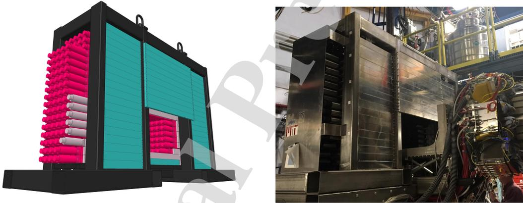
Figure 13: (left) CAD drawing of the downstream side of BAND and its frame. The lead wall is shown in cyan, the scintillators are in magenta, and the support frame is in black. (right) Photograph of the downstream side of BAND installed in Hall B. The reflective surface in the photograph are the aluminum covers of the lead blocks.
