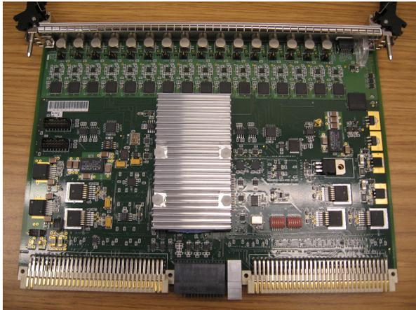
Figure 12: Flash ADC module (FADC250). The 16-channel, 12-bit, 250 MHz digitizer in VXS format is capable of providing information to both the readout chain over the VME bus and the trigger logic over the VXS serial lines.
