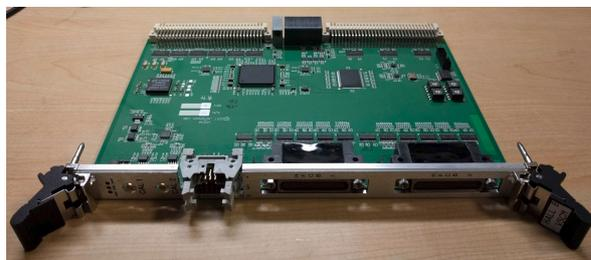
Figure 18: VXS Silicon Readout Module (VSCM). Designed to interface the FSSR2-based Silicon Vertex Tracker detector front-end to the CLAS12 DAQ system.
