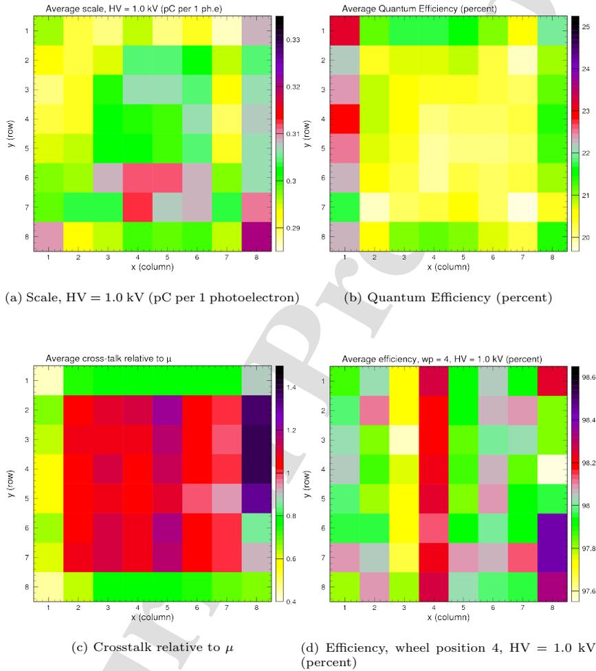
Figure 29: Two dimensional plots showing the average (a) scale, (b) quantum efficiency, (c) crosstalk relative to  $\mu$ , and (d) efficiency as a function of pixel location. The results are averaged for the full set of 399 Hamamatsu H12700 MaPMTs. The pixel numbers increment from left to right, top to bottom, with pixel #1 in the top left corner.
