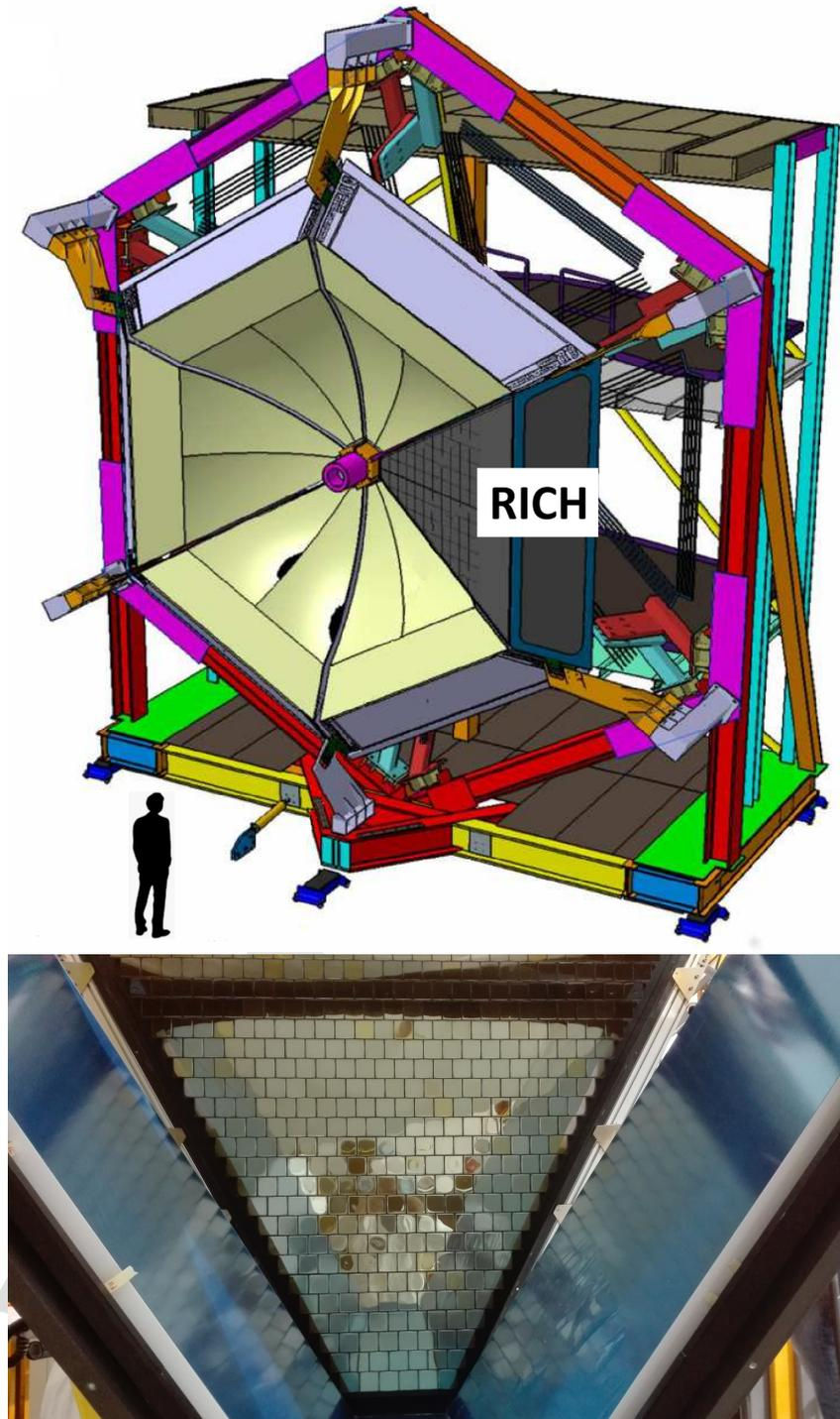
Figure 1: Top: The part of the CLAS12 detector with the RICH covering one out of six sectors. Bottom: the photomatrix of multianode photomultipliers and the mirror system.
