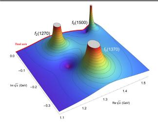
FIG. 2.  $|F^{00}(s, t = 0)|$  obtained from the  $F^{00}$  FDR, using as input the CFD in [56], analytically continued by means of continued fractions. Note the  $f_2(1270)$  pole between the real axis and the  $f_0(1370)$  pole, and the  $f_0(1500)$  pole nearby.
