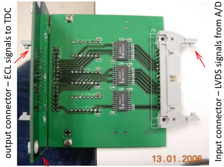
FIG. 5.6: Photograph of one level translator card designed for the MAD cards.
