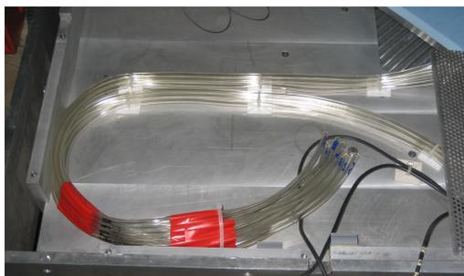
FIG. 5.13: Photograph of the gas output pipes for the SC of the U planes One pipe corresponds to one subgroup of tubes.
