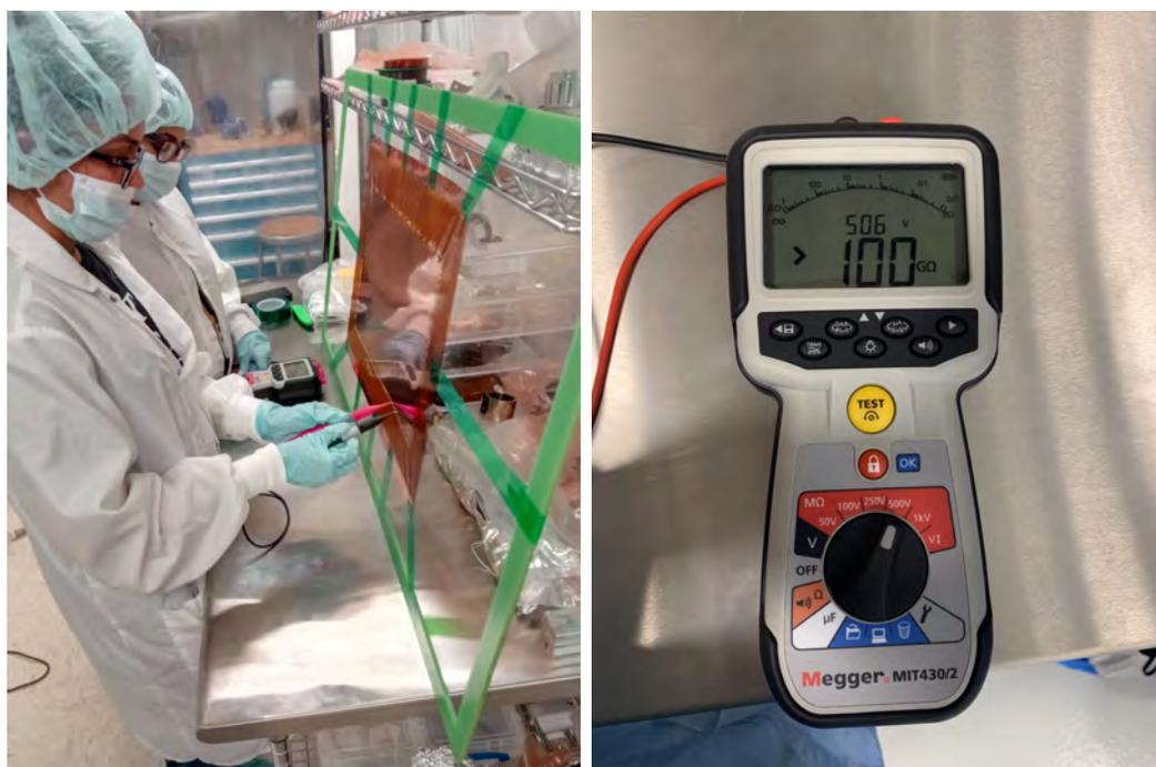
*Figure 4.15.* The performance of pre-stretched GEM foils at high voltages is being tested using the Megger MIT430/2 insulation tester.
