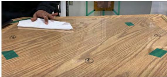
*Figure 4.21.* Cleaning the Plexiglas base with a piece of anti-static tacky cloth.
