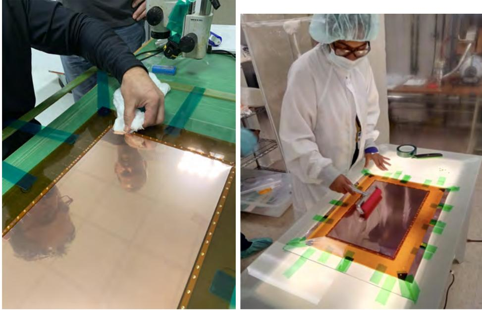
*Figure 4.27.* Pressing down the drift foil onto the adhesive strips using the tacky cloth and cleaning the drift foil using tacky roller after final pre-stretching.
