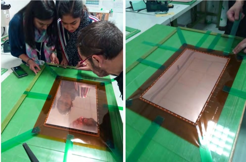
*Figure 4.26.* Placing the drift foil onto the frames while on green canvas and adjusting and pre-stretching the drift foil using green tape
