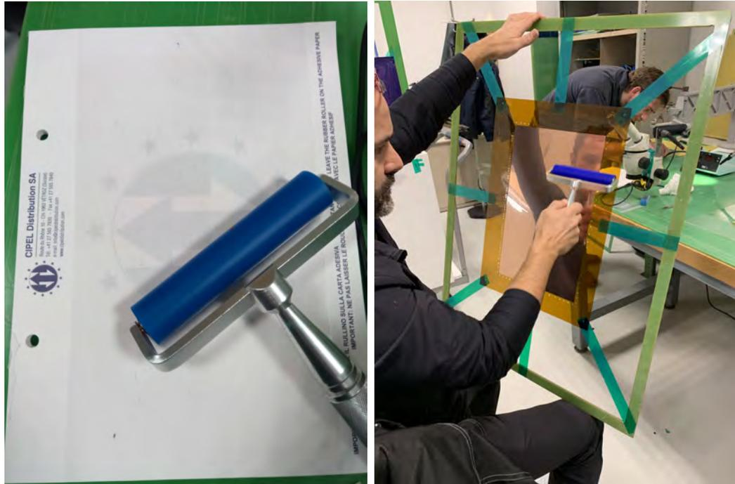
Figure 4.25. Tacky roller (left) and cleaning of the drift foil using tacky roller.
