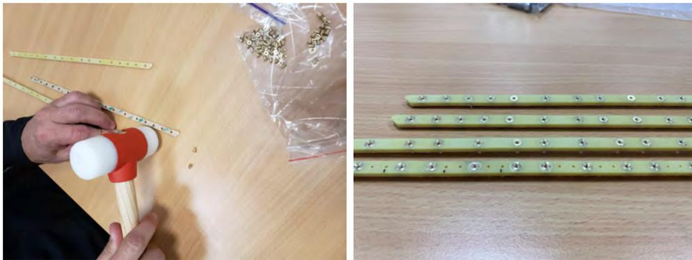
*Figure 4.19.* Hammering of inlay nuts into the inner frame A (Left) and non-adhesive side of prepared frame A (Right).
