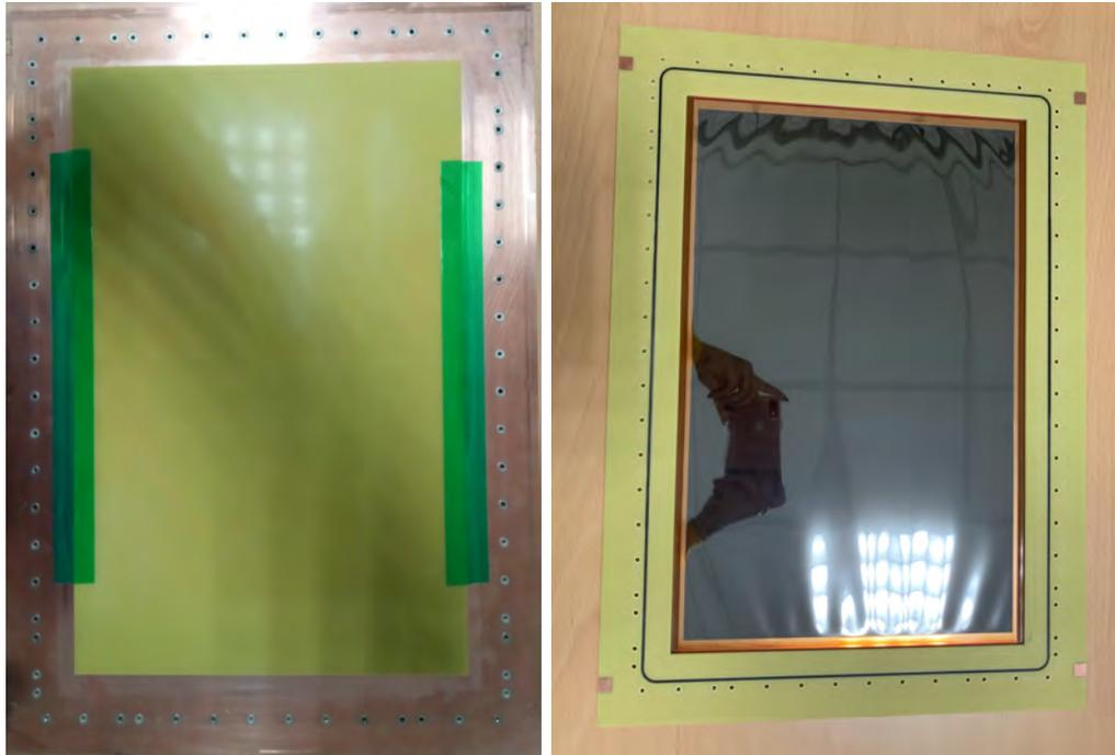
*Figure 4.17.* Top side of top cover with fixed inlay nuts (Left) and bottom side of top cover with embedded o-ring (Right).
