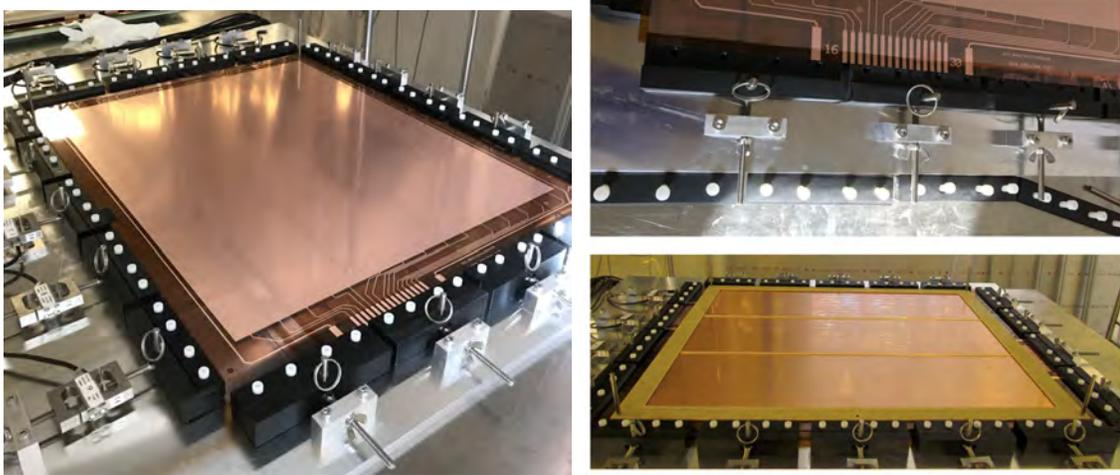
*Figure 4.1.* Mechanical stretching of 50 x 60 cm<sup>2</sup> GEM foils made for a SBS by UVA - Left: Stretched GEM foil using a mechanical system on four sides. Right: Top figure shows the close-up of the mechanical system and bottom figure shows the GEM foil after gluing on to the spacer frame.
