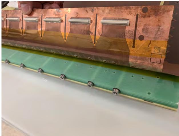
*Figure 4.51.* Placement of M6 screws through openings where horizontal screws sit (Left).
