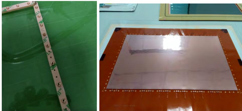
*Figure 4.23.* Extra holes on one side of inner frame A bar and on the drift foil for HV connections.
