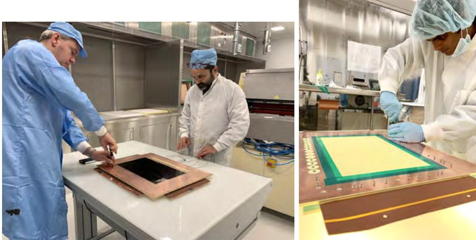
*Figure 4.50.* Closing the chamber by inserting screws through bottom cover.
