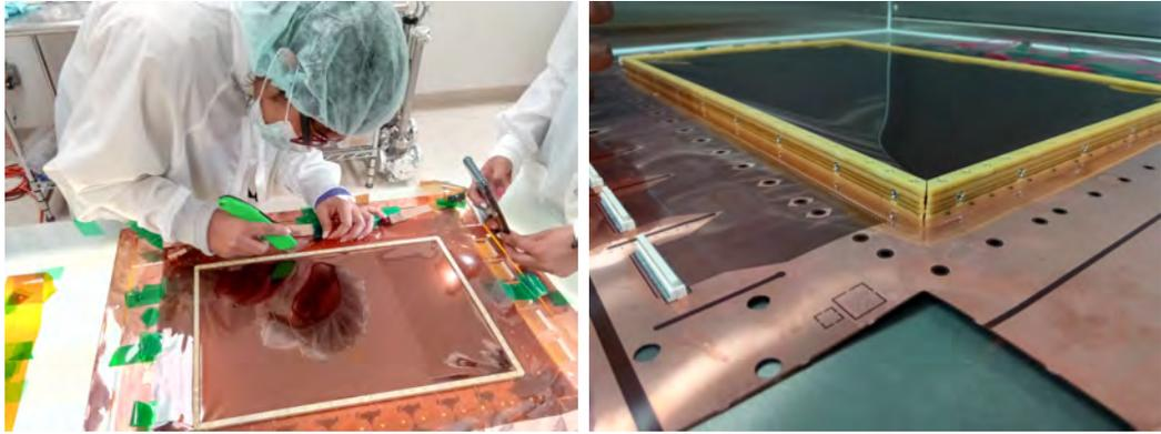
*Figure 4.42.* The GEM foil stack after cutting off excess foil.
