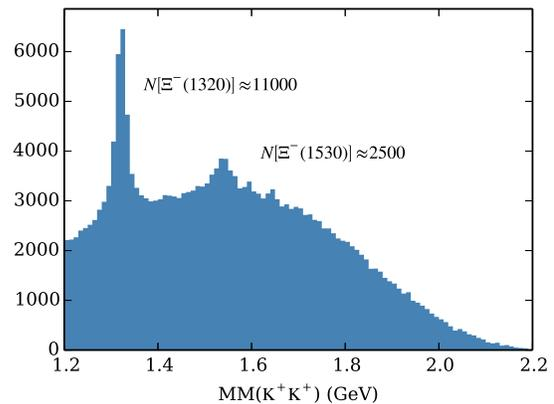
FIG. 2. Missing mass off ( $K^+K^+$ ) showing the  $\Xi$  spectrum above a smooth background, summed over all angles and all  $E_\gamma$ . The two lowest-lying states are shown along with their approximate yields. The missing-mass resolution of the CLAS detector is about 0.01 GeV.
