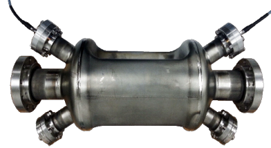
Figure 3. “RF dipole” crab cavity developed by ODU.
