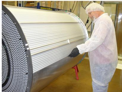
Figure 6: Straw-tubes in layer 28, with one half of the outer shell in place.
