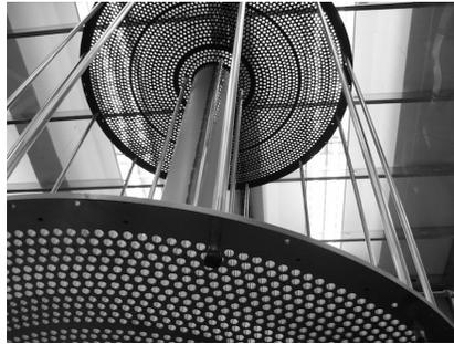
Figure 2: CDC frame prior to the installation of the straw-tubes.
