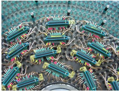
Figure 11: Hookup wires and transition boards.
