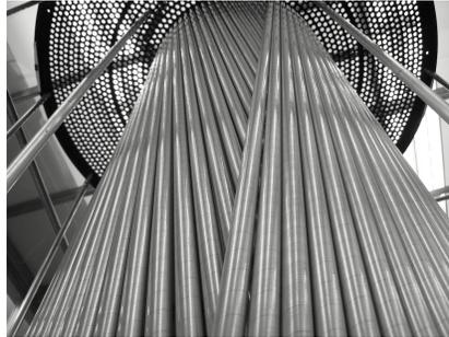
Figure 5: Straw-tubes in stereo layers 8 and 9.
