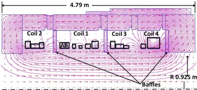
Fig. 2. Half solenoid cross section at 45° to the vertical with subcoils, the relative changes in the magnet flux density field profiles in the magnet, and yoke are shown for Hall D magnet configuration.
