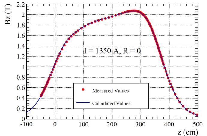
Fig. 3. Calculated and measured magnet flux density plot along the magnet bore at 1350 A.
