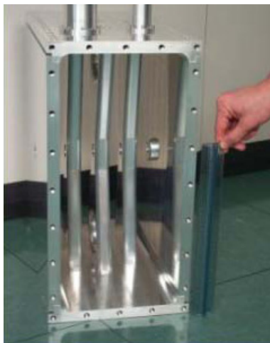
Fig 5: Ladder cavity under construction at LNL [34].
