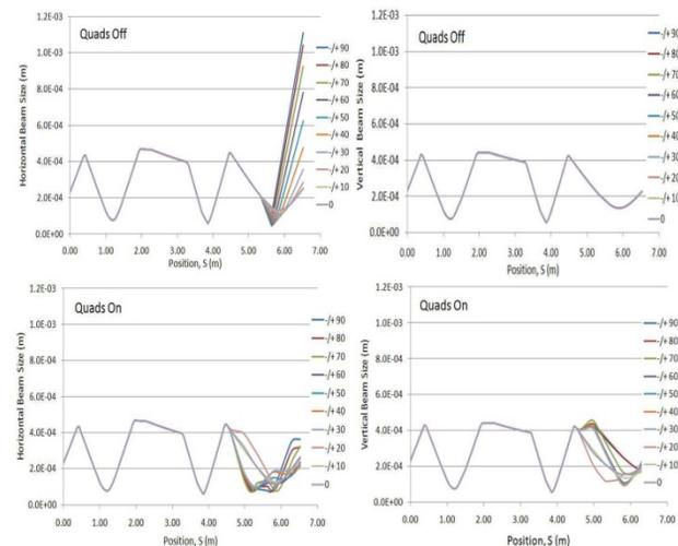
Figure 4: RMS beam size (horizontal/vertical) vs. Wien filter spin angle ( $\pm 90^\circ$  in  $10^\circ$  increments) without (upper) and with (lower) quadrupole correction.
