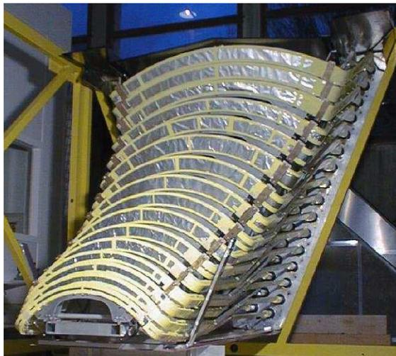
FIG. 3.12: Photograph of FPDs for a single octant. Eight such octants existed and were mounted together on a Ferris wheel that can be seen in Figure 3.11.
