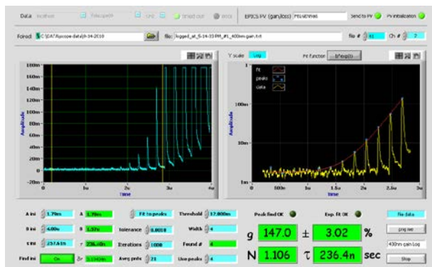
Figure 5: FEL gain data acquisition software. Left: linear scale; right: logarithmic scale
