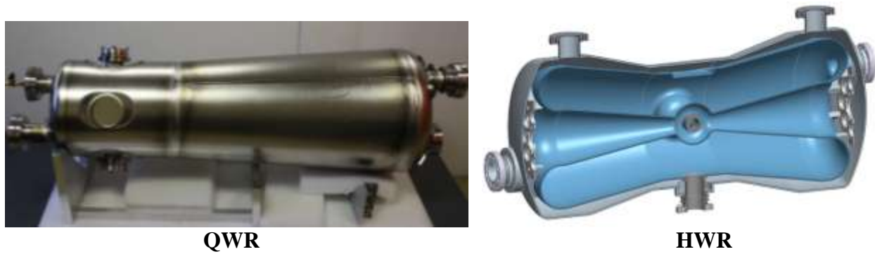
Figure 5.9: Superconducting cavities for the MEIC linac.
