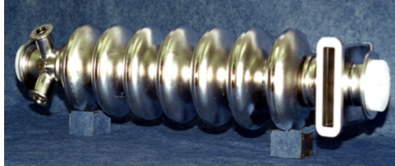
FIG. 5: The 12 GeV upgrade CEBAF single 7-cell cavity. It has 70 cm effective length with 1497 MHz RF with 19 MV/m energy gain.
