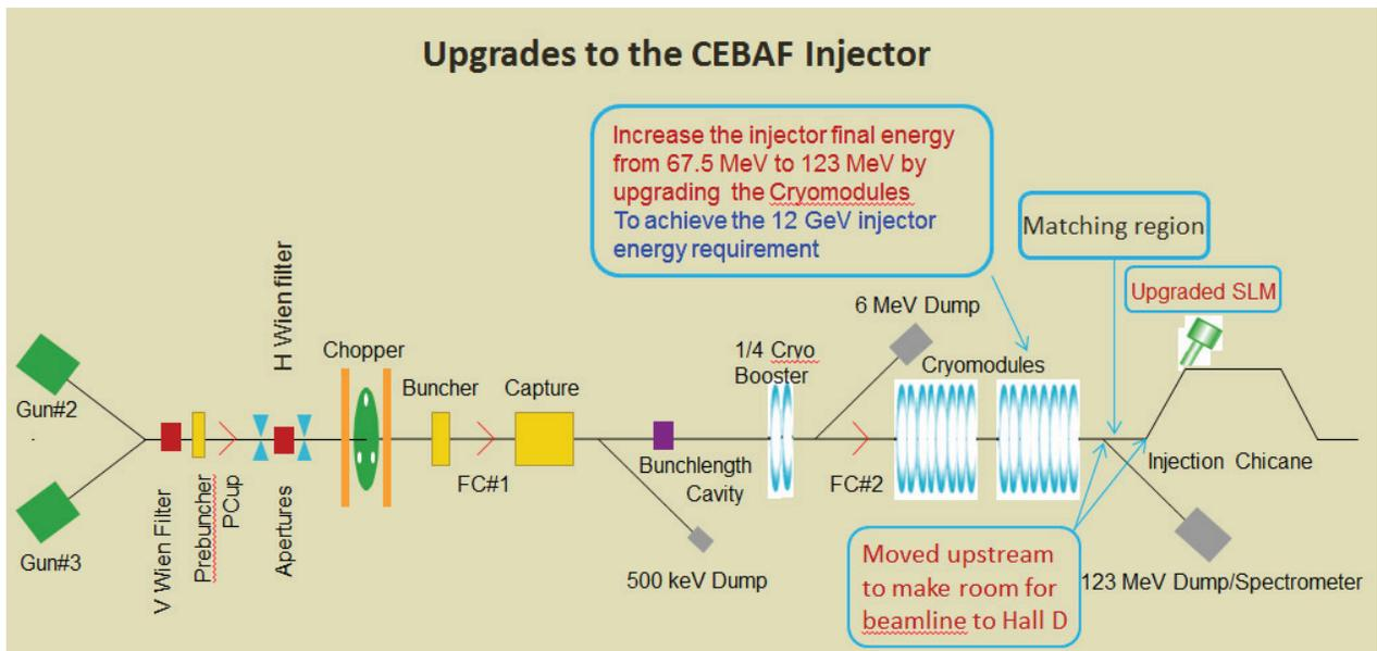
Figure 1: Upgrades make the injector compatible with the 12 GeV CEBAF (not to scale).
