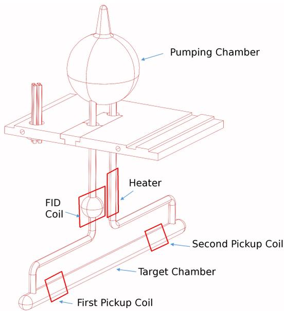
Figure 6-26: Set up for convection flow test.
