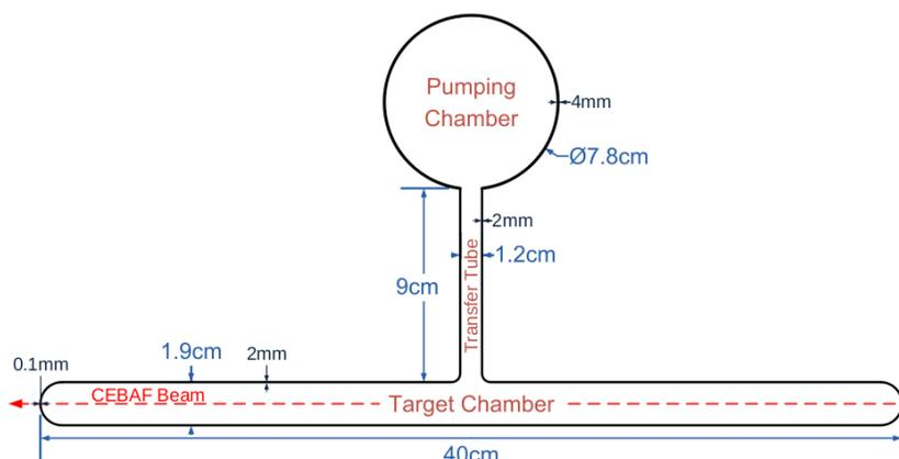
Figure 6-9: Geometry of a typical polarized  $^3\text{He}$  Cell used by Transversity experiment[168].
