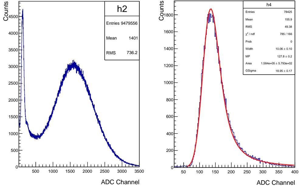
Figure 4-1: A typical ADC signal from one PMT of Gas Cherenkov.
