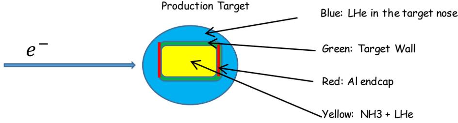
Figure 4-21: NH<sub>3</sub> target in the target nose. The target nose is 4.20 cm in diameter, the target cell length is 2.83 cm, each of the aluminum endcap has a thickness of 0.7 mil.
