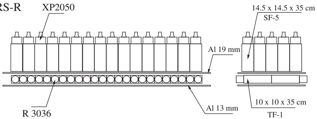
Figure 3-27: The electromagnetic calorimeters in the HRS[92]. The scattered particles direction is from bottom to top.
