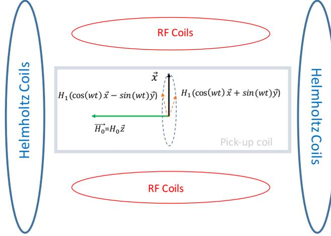
Figure 6-11: The field setup for NMR system.
