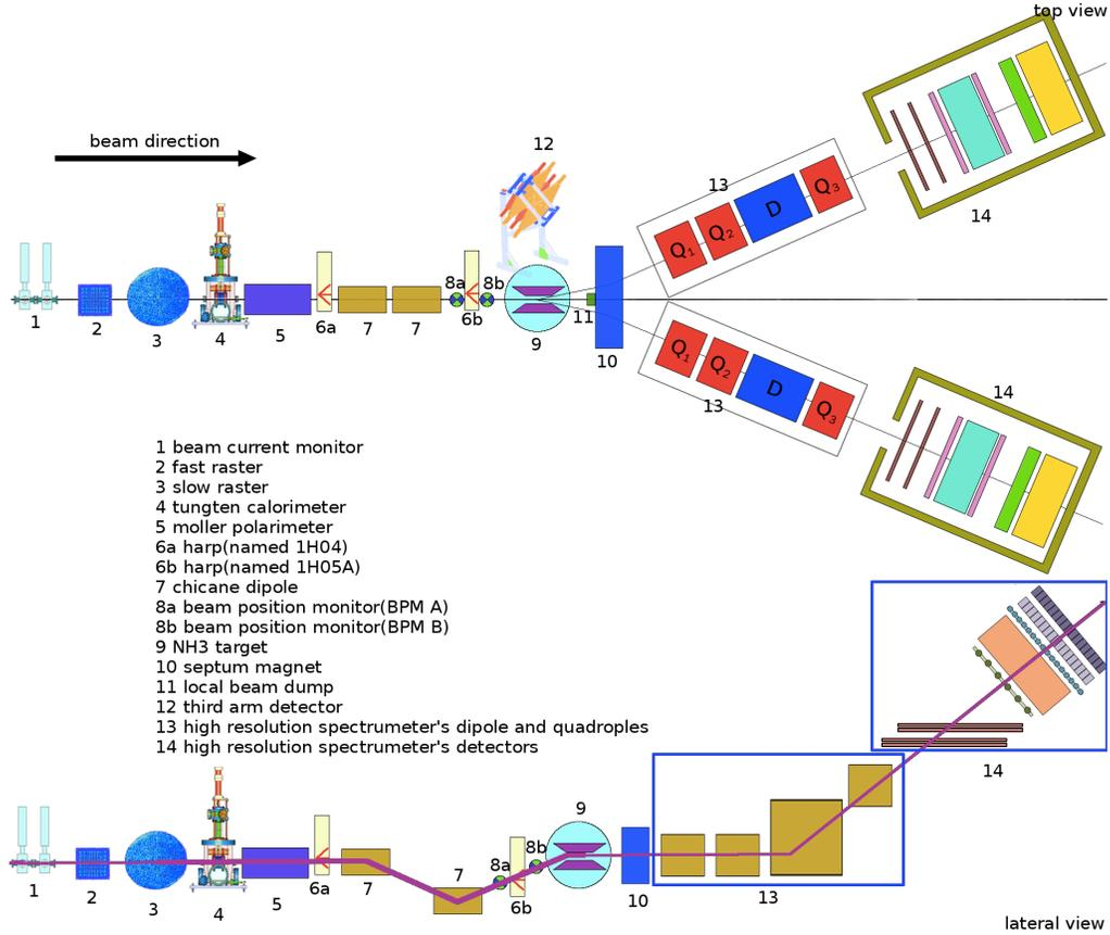
Figure 3-3: Schematic of Hall A during E08-027[93].
