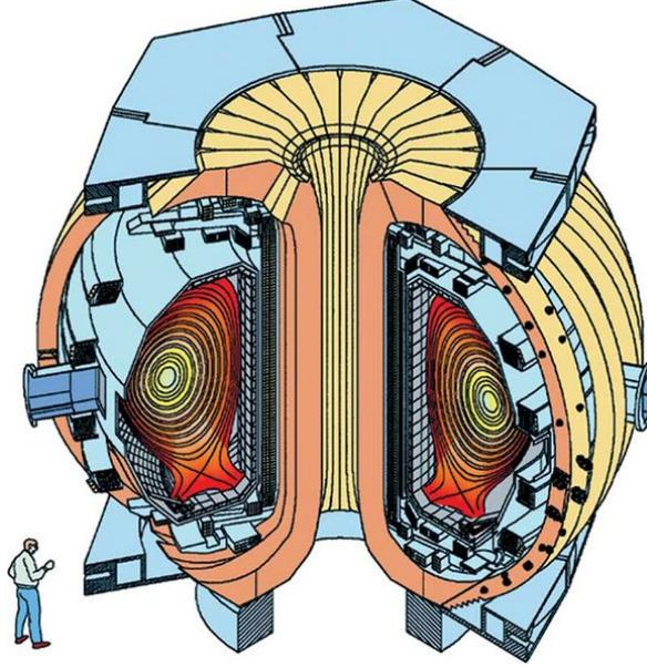
Figure 7-8: DIII-D tokamak in San Diego operated by GA[206]. Its a research-scale tokamak with room temperature coils. Its major radius  $R_0$  is 1.67 m, minor radius is 0.67 m, plasma volume is  $30 \text{ m}^3$ . The toroidal field at  $R_0$  is 2.1 T. Plot reproduced from [207].
