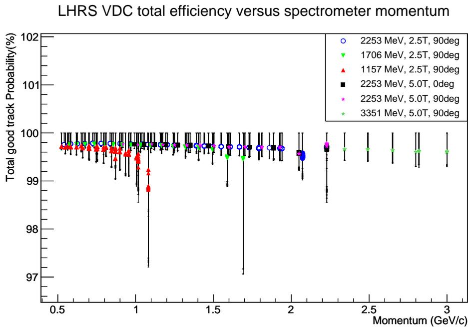
Figure 4-19: LHRS VDC efficiency with systematic uncertainty
