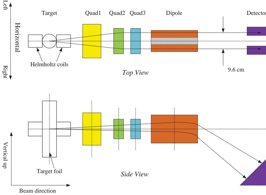
Figure 3-9: Schematic diagram of the Møller polarimeter[92, 104].
