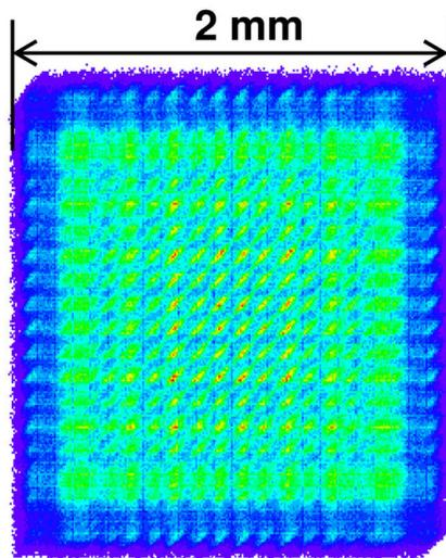
Figure 3-5: Fast raster pattern, produced from the magnet current signal[100].
