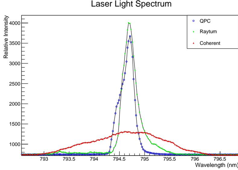
Figure 6-3: Comparison of laser wavelength spectrum between vendors. Coherent is the broad-width diode laser (FWHM $\approx$ 1.5 nm) while QPC and Raytum are new narrow-width ones (FWHM $\approx$ 0.25 nm).
