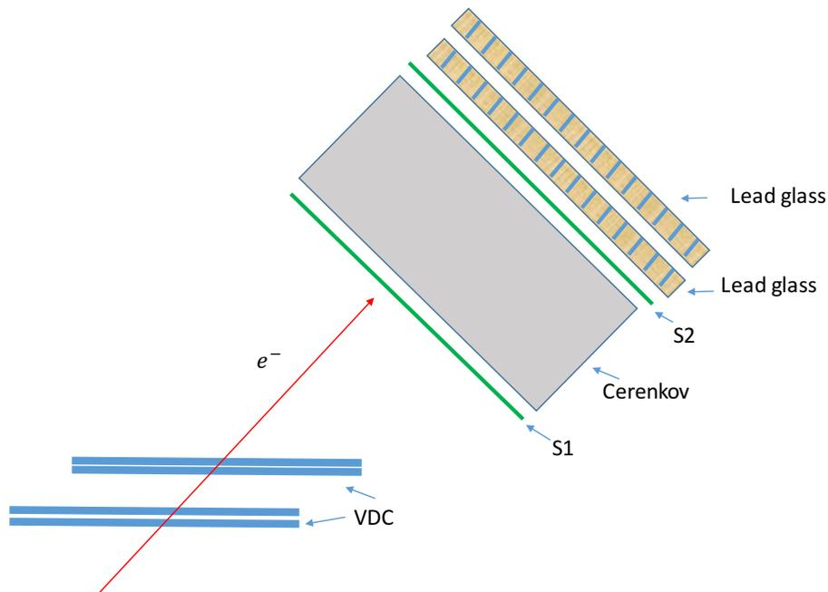
Figure 3-21: Detector package for HRS.
