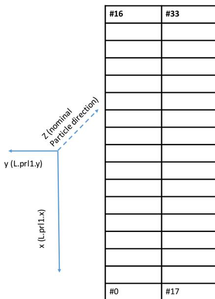
Figure 4-11: The arrangement of the blocks in one layer of lead glass (pion rejector).
