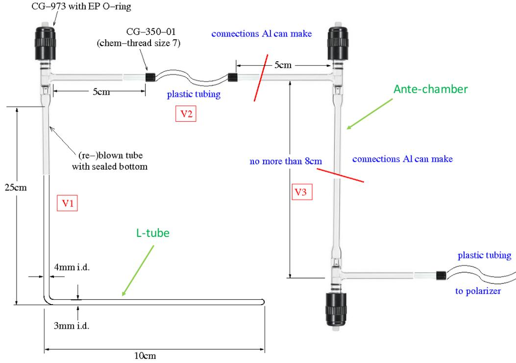
Figure 7-28: The L-tube connected with an ante-chamber.
