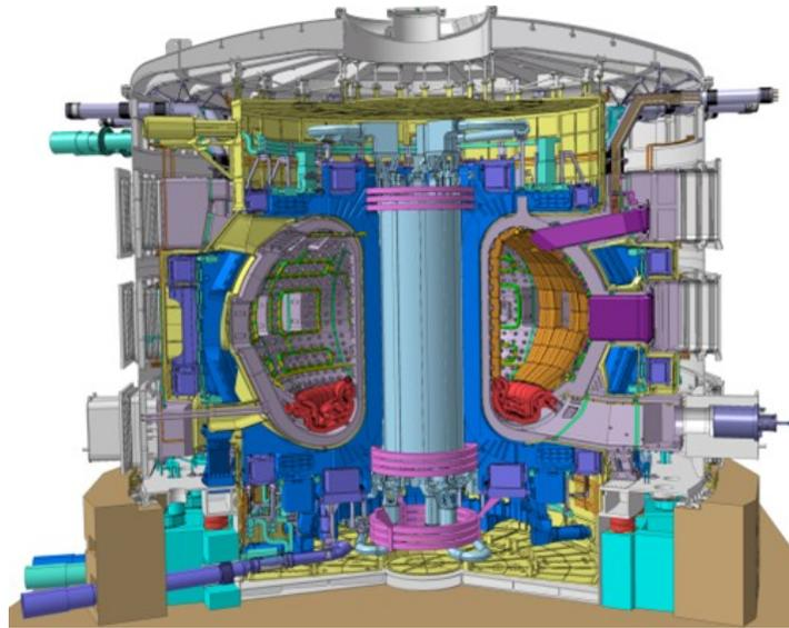
Figure 7-5: ITER Tokamak is currently being built in southern France in the framework of a collaboration between China, Europe, India, Japan, Korea, Russia and the USA. It will use superconducting coils. Its major radius  $R_0$  is around 6.2 m, minor radius is 2.0 m, and its plasma volume is  $820 \text{ m}^3$ . The toroidal field at  $R_0$  is 5.3 T. Plot reproduced from [200].
