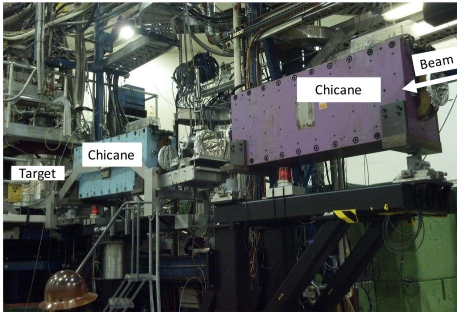
Figure 3-10: Chicane dipole magnets upstream of the target.
