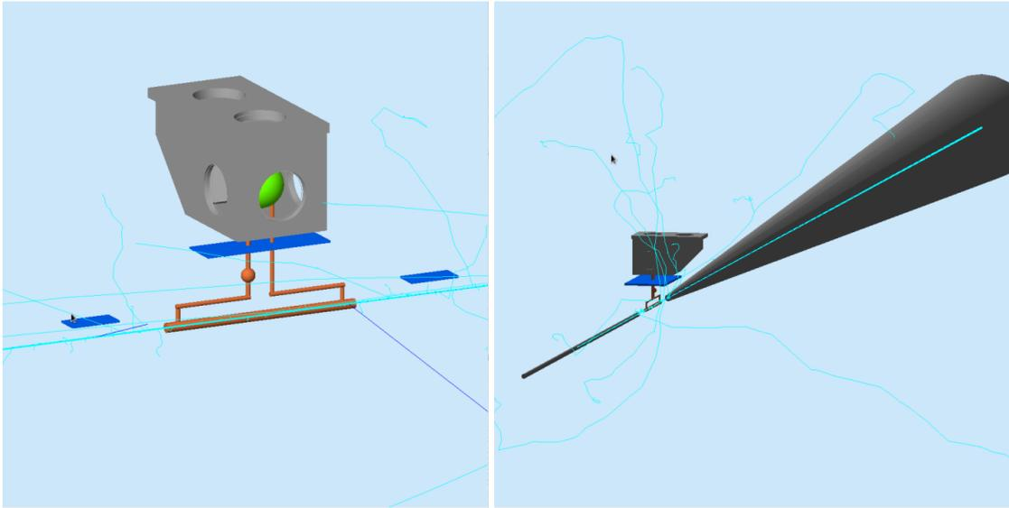
Figure 6-36: Simulation setup for radiation shielding study. The left plot shows the setup including the  $^3\text{He}$  target, oven, collimators and a piece of shielding plate of lead, while the right plot shows the setup with the beam line.
