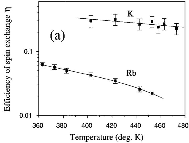
Figure 6-5: Spin exchange efficiency comparison (note logarithmic scale) for  $^3\text{He}$ -Rb (7.0 amagat of  $^3\text{He}$ ) and  $^3\text{He}$ -K (6.9 amagat of  $^3\text{He}$ ) versus temperature[164].
