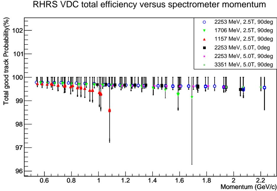
Figure 4-20: RHRS VDC efficiency with systematic uncertainty
