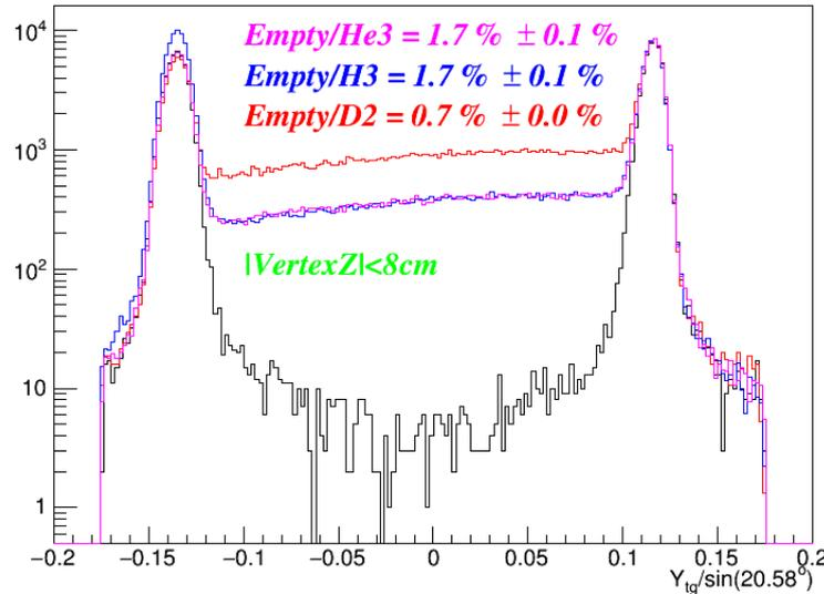
CENTER Image: Shown are the tritium, He, D target data as compared to running on an empty cell (black). The tritium and other gas targets are clearly visible between the aluminum entrance and exit windows of the target cell.
