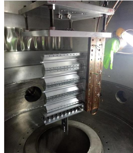
RIGHT Image: The target cell stack during installation in the Hall A scattering chamber.
