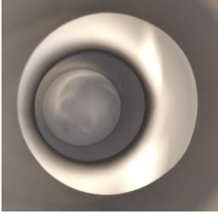
Figure 1: A picture of SC-IB interior after \text{Nb}_3\text{Sn} coating.
