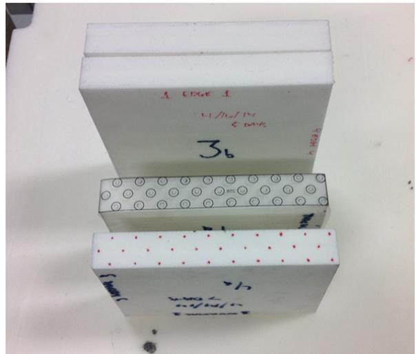
Fig. 19: Foam pieces marked for an approximately 22.5% epoxy coverage pattern.
