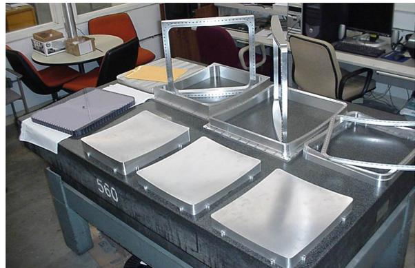
Fig. 6: Tooling set for the manufacture of mirror facet #3.
