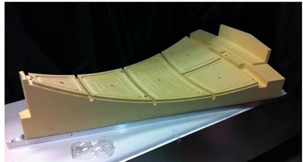
Fig. 26: One of the 12 polyurethane half-sector holding tables.
