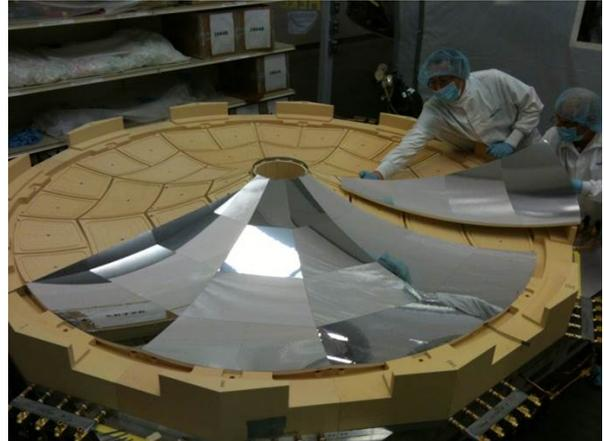
Fig. 29: Partially assembled combined HTCC mirror.
