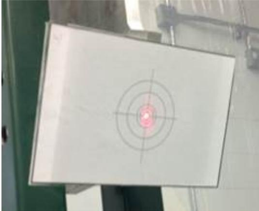
Fig. 24: Light collection pattern on the focal plane. The laser beam is rasterized in the plane crossing the mirror covering polar and azimuthal angles in the range of  $\theta = 5^\circ - 12.5^\circ$  and  $\phi = 0^\circ - 30^\circ$ , respectively.
