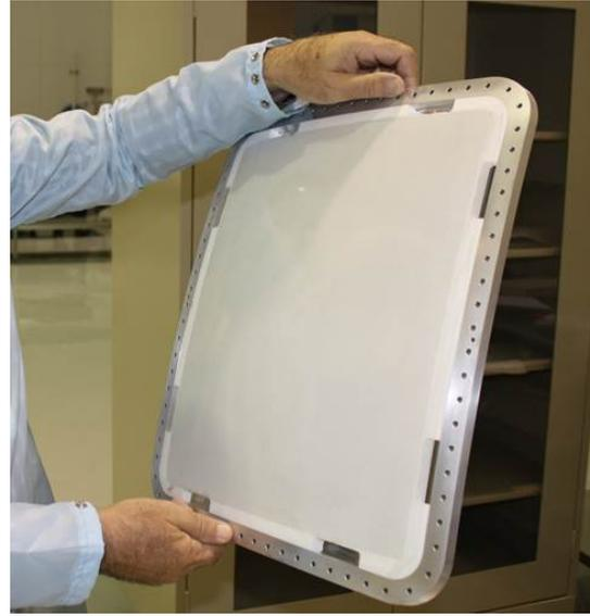
Fig. 12: Sandwiched mirror facet after gluing components as shown in Fig. 11.
