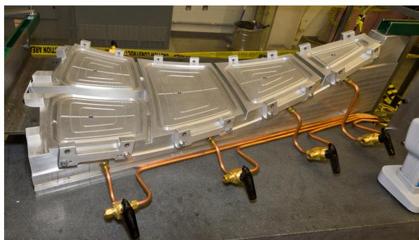
Fig. 18: High-precision table for the assembly of the half-sector mirrors.
