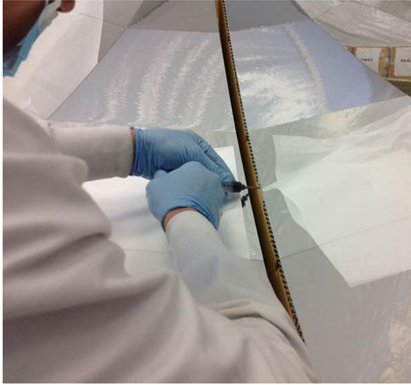
Fig. 31: Application of the epoxy glue on the side of the separated halves of the combined mirror.
