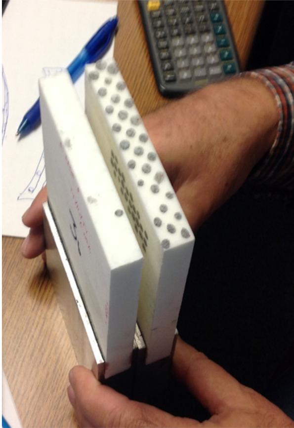
Fig. 21: Broken epoxy glue joint between two PMI foam pieces.
