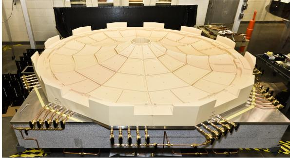
Fig. 27: All 12 half-sector vacuum tables assembled on their 1-in aluminum plates placed on the granite table.
