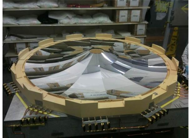
Fig. 32: Fully assembled combined HTCC mirror.
