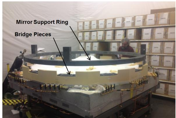
Fig. 33: Supporting elements ready to be attached to the combined mirror. The mirror is covered with soft paper towels to protect the working surface from debris.
