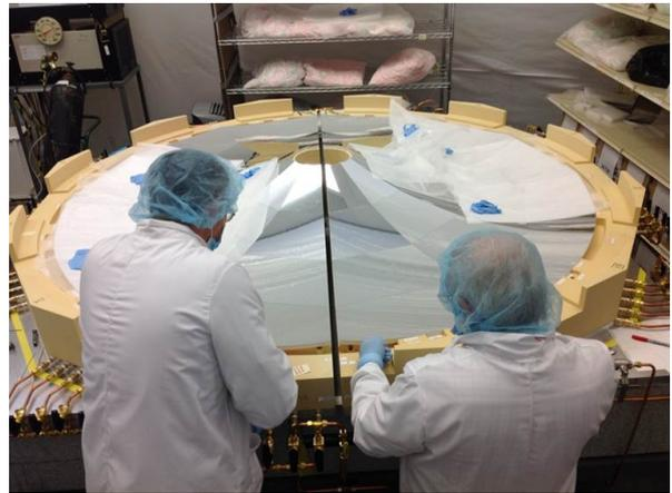
Fig. 30: Separated halves of the combined mirror before final gluing.
