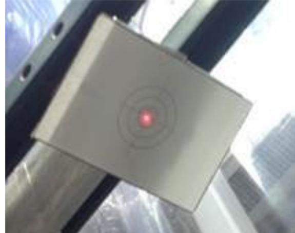
Fig. 25: Light collection pattern on the focal plane for the mirror covering polar and azimuthal angles in the range of  $\theta = 27.5^\circ - 35^\circ$  and  $\phi = 0^\circ - 30^\circ$ , respectively.
