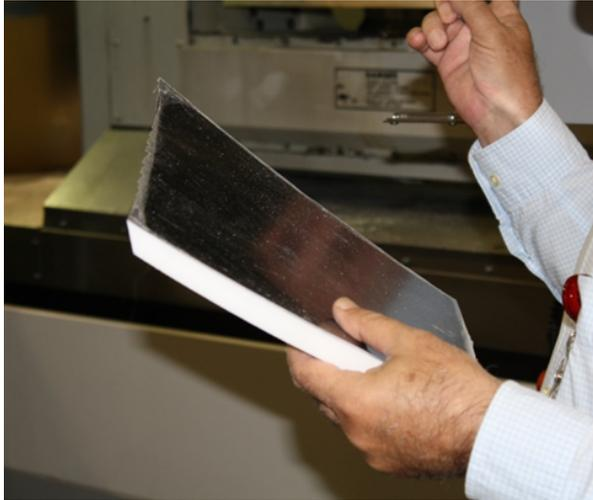
Fig. 15: Completely trimmed mirror facet #3 covered with protection film.
