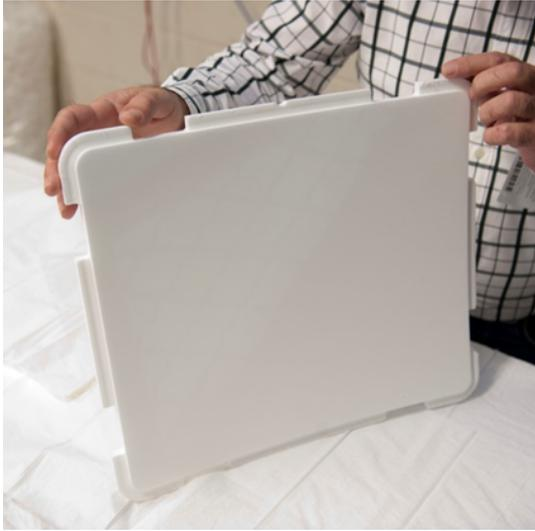
Fig. 10: A completed foam substrate that forms the core of the mirror facet.
