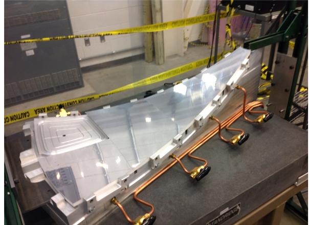
Fig. 22: Partially assembled half-sector mirror. The left facet of the last largest mirror is not installed yet.
