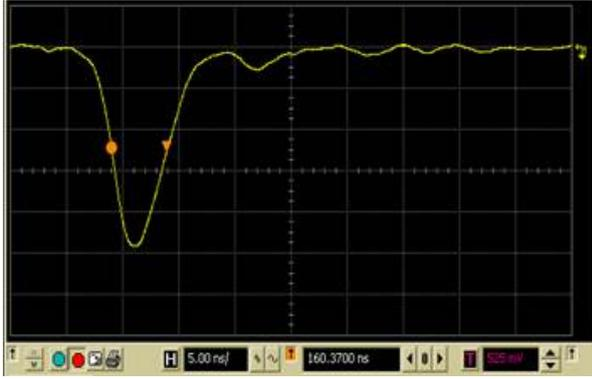
Fig. 51: Typical output signal provided by a passive HV-divider.
