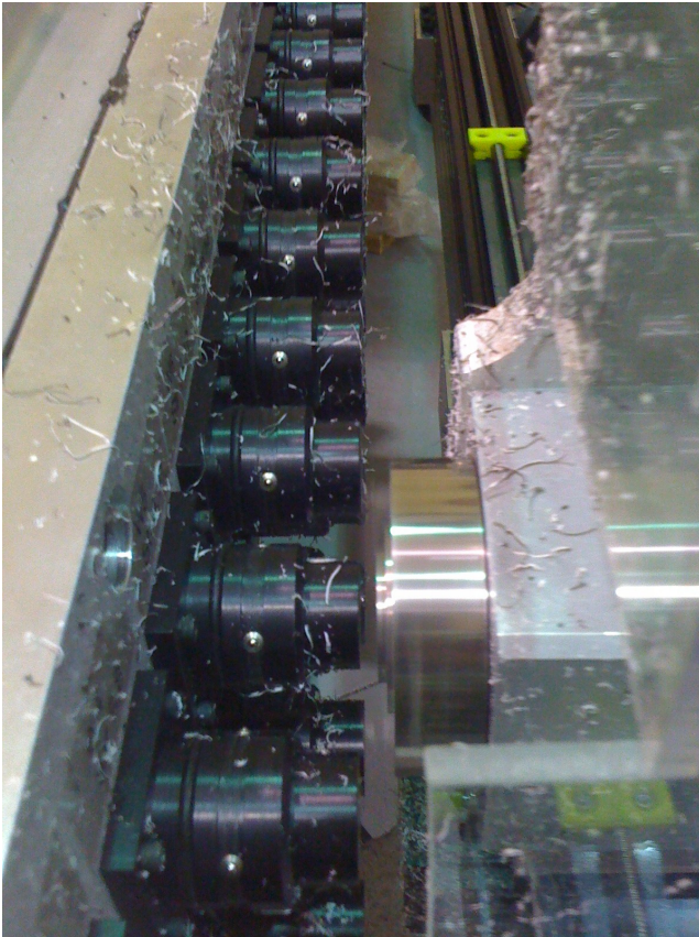
Figure 15: Fly cutter of fiber cutting machine making an initial milling pass of PCAL WLS fiber bundles.
