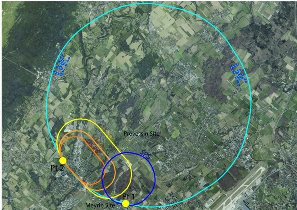
**Figure 8.46:** Racetrack options proposed for LHeC at Point 2 of the LHC. The color coding illustrated different options with 1/3, 1/4 and 1/5 of the LHC circumference, resulting in different electron beam energies.
