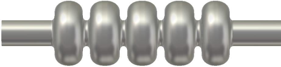
**Figure 8.14:** Bare 802 MHz five-cell cavity design (RF vacuum) with a 130 mm iris and beam tube aperture.
