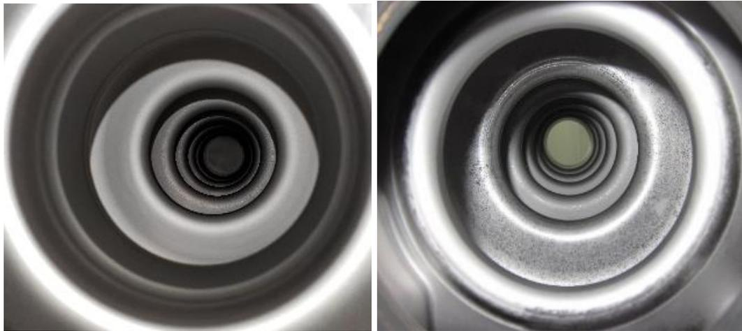
Figure 4.47: Pictures C75-RI-NbSn1 taken from the bottom [left] and the top [right]. The coating looks non-uniform from the top.
