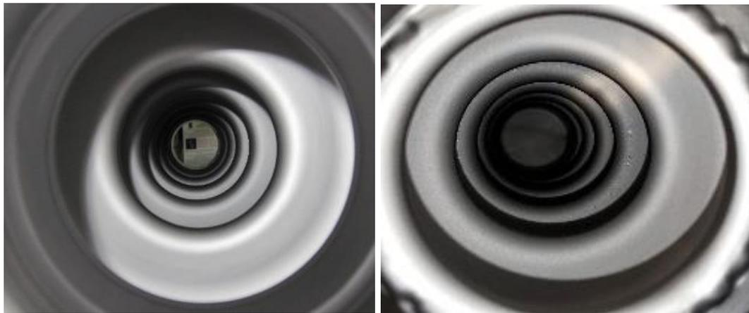
Figure 4.48: Pictures from C75-RI-NbSn2 taken from the bottom [left] and the top [right]. The coating looks mostly uniform from each side.
