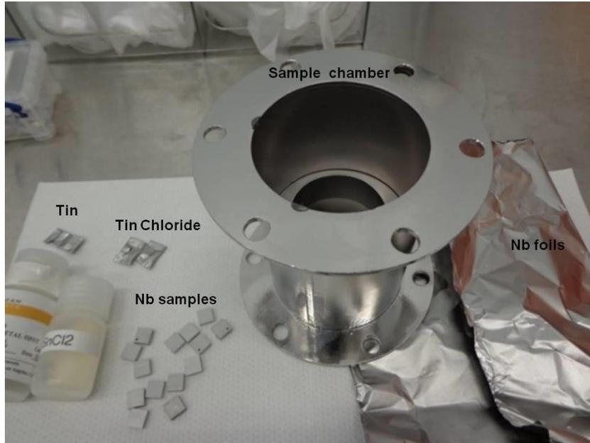
Figure 1.9: Sample chamber, samples, tin and tin chloride packages, and Nb foils before setting up for the coating. The coating chamber of the furnace is not shown.
