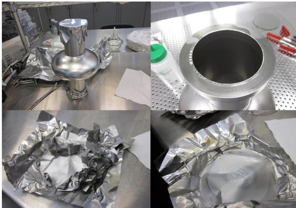
Figure 4.1: Cavity C3C4 after the coating run. Note discoloration on the NbTi cavity flange (b) and 'tin' droplets on the niobium foil from the cavity top flange (d).
