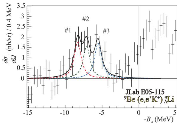
FIG. 2. A fitting result on the  ${}^9\text{Be}(e, e'K^+)_{\Lambda}{}^9\text{Li}$  spectrum by three Voigt functions. A distribution of the accidental coincidence events that was obtained by the mixed event analysis (Fig. 1) was subtracted from the original spectrum.
