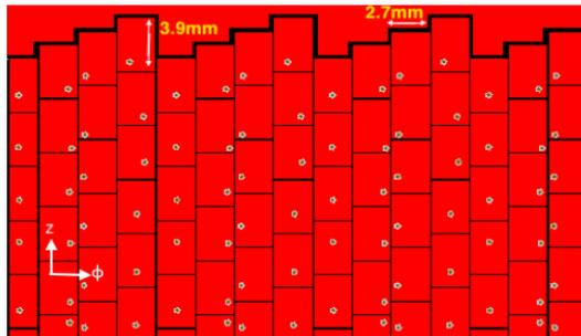
FIG. 17: Padboard readout pattern in the BONuS12 experiment.
