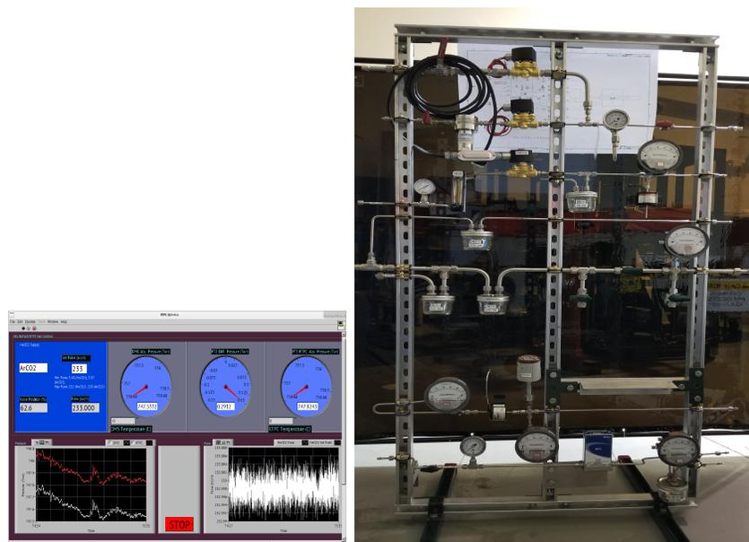
FIG. 49: BONuS12 gas panel with various sensors and safety components approved by the Hall B engineering (right); and control and monitoring of the drift gas (left).
