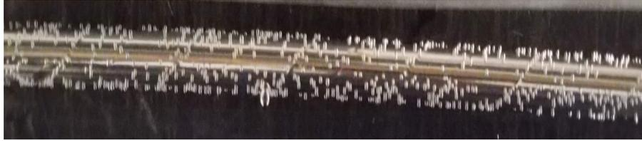
FIG. 48: Leakage of Helium from the double sided aluminum coated straw visualized as bubble under water.
