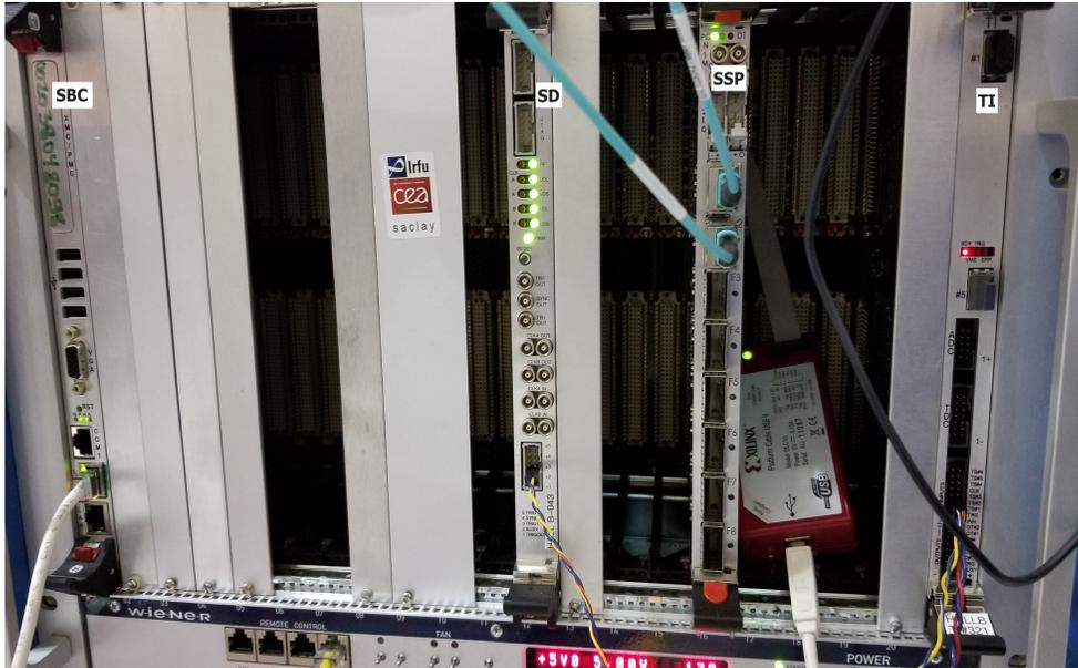
FIG. 55: Components of the CLAS12 BEU consisting of SBC, TI, SSP, SD. Twisted cable with crimp connector are connected to the TI and SD front panel for standalone operation.
