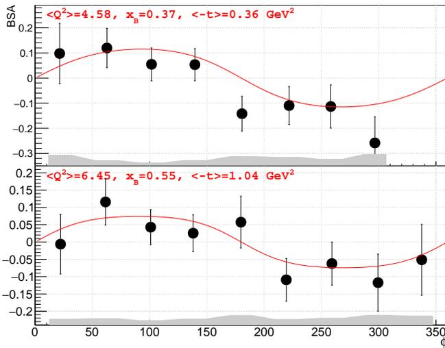
FIG. 5. Beam spin asymmetry as a function of  $\phi$  for two representative kinematic bins. The vertical error bars show the statistical uncertainty of each point. The gray bands represent systematic uncertainties of the BSA measurements. The red lines show the fit with functional form of Eq. (1).
