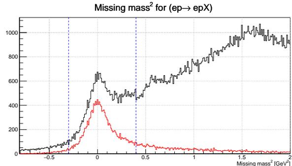
FIG. 2. Distributions of missing mass squared of the  $epX$  system before (black line) and after (red line) application of the exclusive constraints. The blue dashed lines represent the cuts on  $MM_{epX}^2$  that were also used for final exclusive  $\bar{e}p \rightarrow e'p'\pi^0$  event selection.
