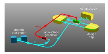
**Figure 1:** Radioactive cesium-137 ions created by bombarding a block of uranium carbide with energetic electrons are directed to a fixed location in an electron storage ring. Electrons circulating in the ring scatter from the cesium target and are recorded by a magnetic spectrometer, or "femtoscope," allowing the properties of the cesium nuclei to be reconstructed.
