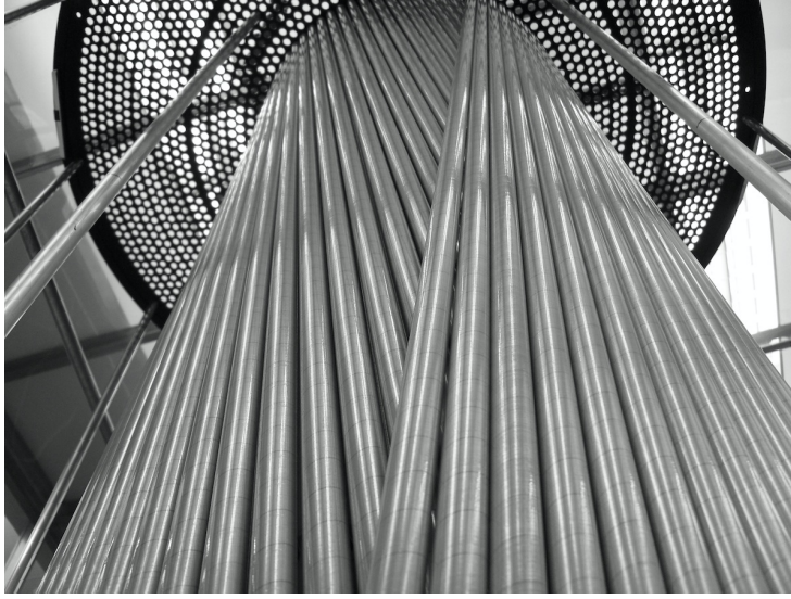
FIG. 2.11: Image of the straws of the Central Drift Chamber during construction [38]. The off-angle orientation of the straws is demonstrated here.
