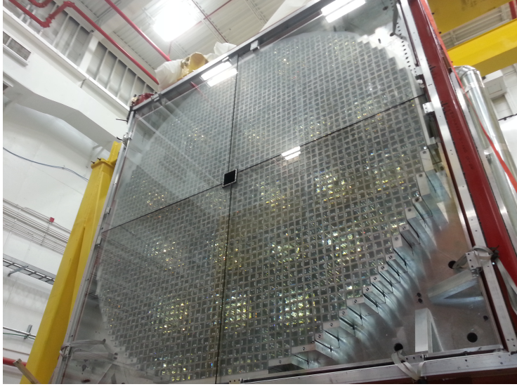
FIG. 2.14: An image of the interior of the Forward Calorimeter where the grid of lead glass blocks can be seen.
