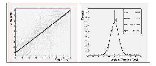
Figure 3-5: The in-plane angle reconstructed in BigBite [deg] vs. the in-plane angle of the proton [deg] as determined from the electron in H(e,e'p) (Left). The difference between the in-plane angle as measured in BigBite and the expected angle from the electron as measured by the HRS (Right).
