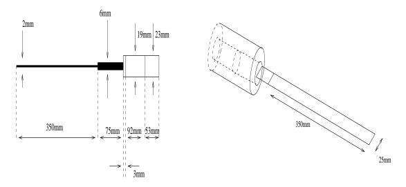
Figure 2-10: A schematic diagram of a single auxiliary plane counter, with the light guide, the PMT and the magnetic shield.
