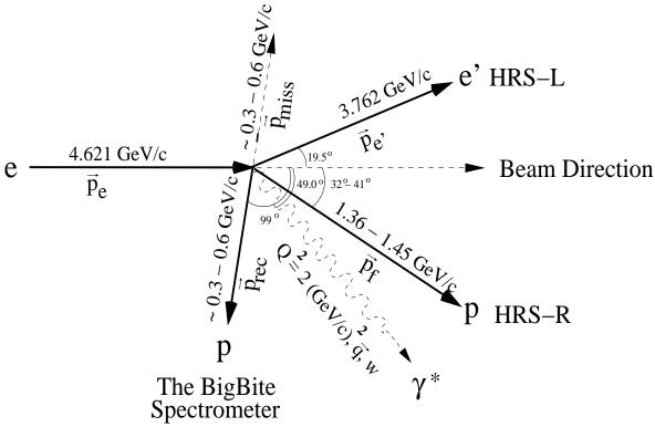
Figure 1-7: A vector diagram of the kinematics of the <sup>12</sup>C(e,e'pp) measurement.
