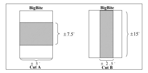
Figure 4-15: The vertical (Left-A) and horizontal (Right-B) angular acceptance cuts defined for the (e,e'p)/(e,e'pp) ratio sensitivity check.
