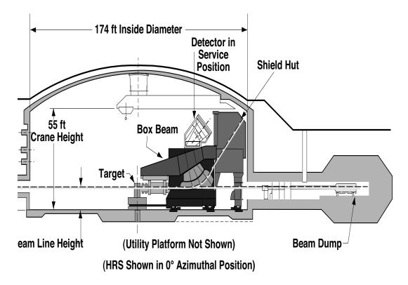
Figure 2-6: Schematic layout of Hall A High Resolution Spectrometer (HRS)
