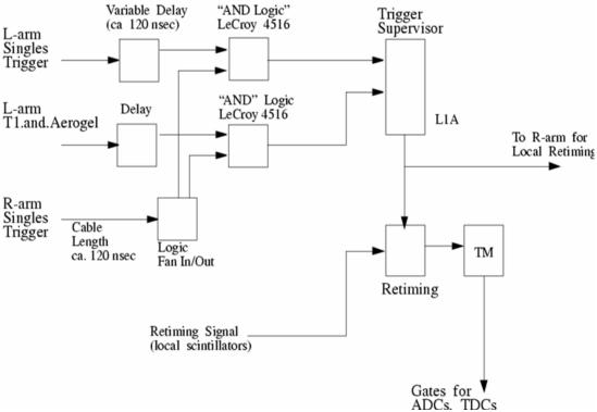
Figure 2-13: Circuit Diagrams of the trigger system.
