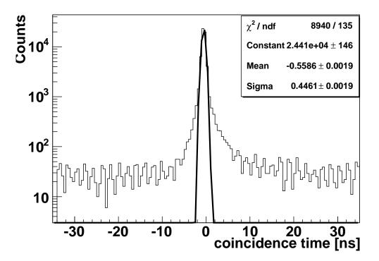
Figure 3-12: The coincidence time between the two HRSs, with a width  $\sigma = 0.4$  ns. The beam structure can be seen with a pulse interval of 2 ns.
