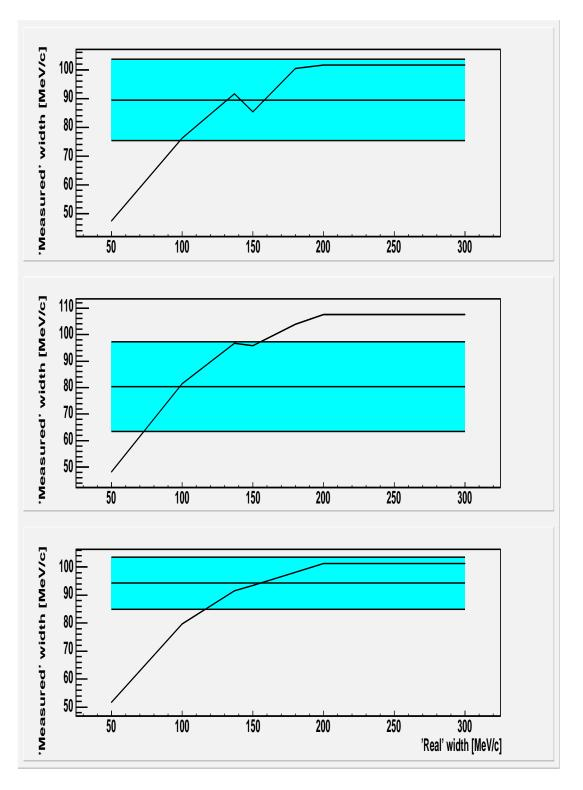
Figure 4-12: 'Measured' vs. 'real' width of the c.m. motion in the scattering plane in the direction of BigBite for K1, K2 and K3 (top to bottom). The curve is a result of the simulation described in appendix B. The middle horizontal line in each plot represents the width from the data. The top and bottom lines define one standard deviation from the central value.
