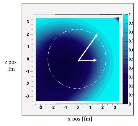
Figure C-6: The combined transparency for the two protons as a function of the interaction point in the nucleus. Notice that here the high momentum proton emerges along the horizontal axis not the vertical axis as in figure C-2.
