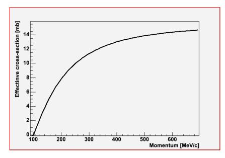
Figure C-3: The effective cross section for low energy protons.
