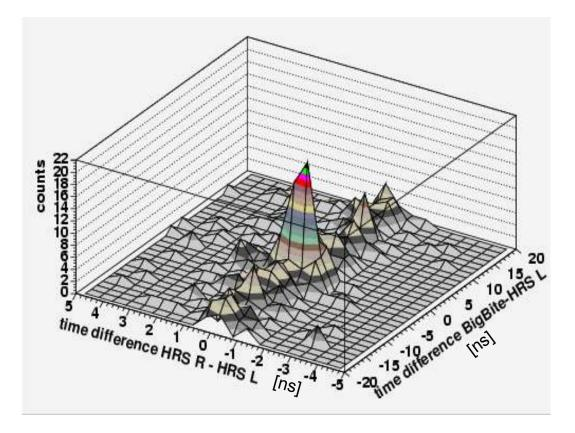
Figure 3-14: Number of counts vs. the time difference between the two HRSs and the time difference between BigBite E-plane and HRS-L.
