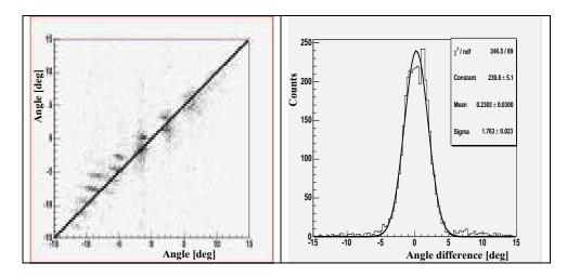
Figure 3-6: The out of plane angle reconstructed in BigBite [deg] vs. the out-of-plane angle of the proton as determined from the electron [deg] (Left). The difference between the out-of-plane angle as measured in BigBite and the expected angle from the electron as measured by the HRS with a typical resolution of sigma=1.5° (Right).
