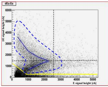
Figure 3-7: The pulse height in the  $\Delta E$  plane vs. the pulse height in the E plane in ADC channels. The lower solid lines represent a low energy deposit areas cut, which are typical to photons and pions. Further PID cuts included a "sleeve" cut, which follows the proton's curve. Deuterium and heavier particles are located in a higher E and  $\Delta E$  energy deposit.
