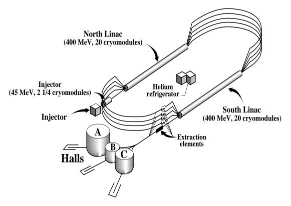
Figure 2-1: Schematic layout of Jlab accelerator.
