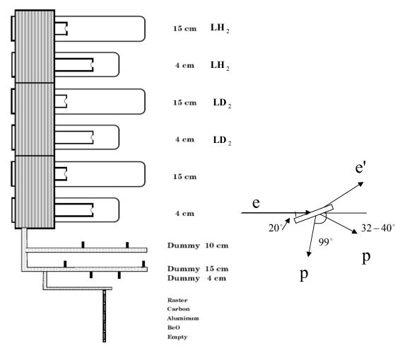
Figure 2-5: Schematic view of the Hall A target ladder for E01-015 and the targets used for the experiment (Left). Schematic view of the tilted carbon target (Right).
