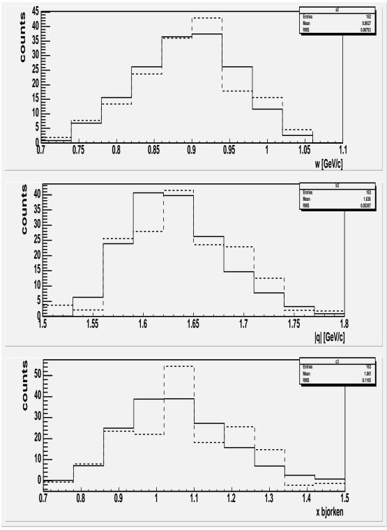
Figure 4-9: The energy transfer distribution [top]. The momentum transfer distribution [middle]. The Bjorken scaling variable  $x_B$  distribution [bottom]. The dashed line represents the measured background-subtracted <sup>12</sup>C(e,e'pp) distribution. The solid line is the <sup>12</sup>C(e,e'p) distributions normalized to the same total number of events. Both curves are after a cut to remove pion and  $\Delta$  production events was applied on the angle of  $\vec{p}_{miss}$ .
