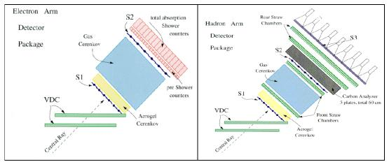
Figure 2-7: A schematic layout of the typical detector packages for the electron (left) and hadron (right) high resolution spectrometers. Note that not all of these detectors were utilized during this experiment.
