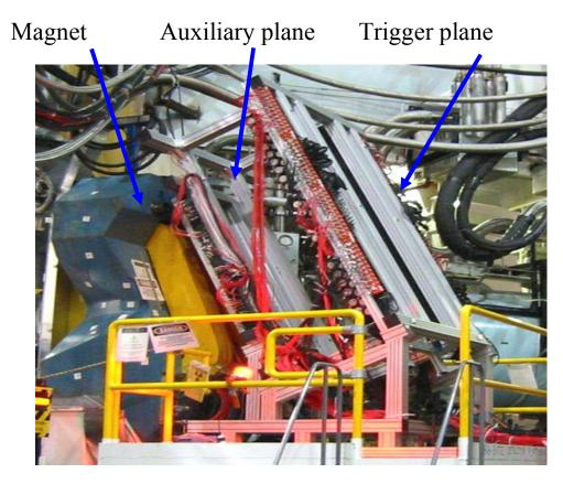
Figure 2-8: A photo of BigBite with the magnet (left) auxiliary (middle) and trigger (right) scintillator detector planes, as set in Hall A for the E01-015 experiment.
