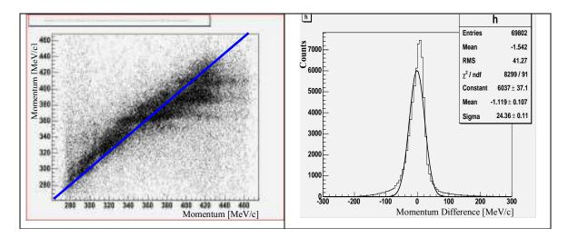
Figure 3-9: The average proton momentum vs. the proton momentum reconstructed from the electron HRS (Left). The difference of the two reconstructed momenta, with a  $\sigma = 25$  MeV/c (Right).
