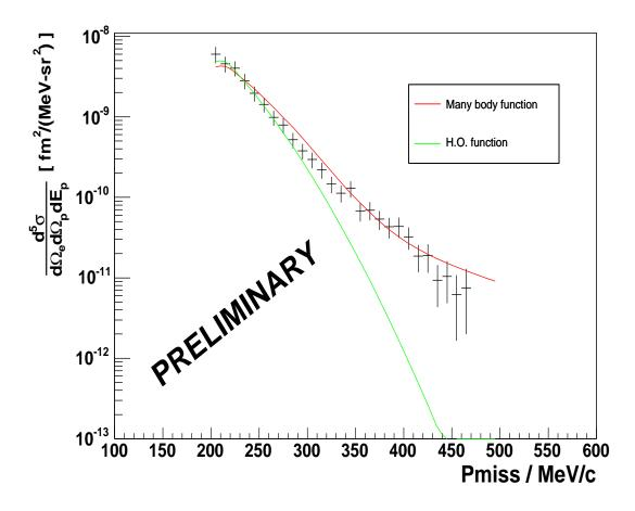
Figure 4-5: Differential Cross-Section for the  ${}^{12}C(e,e'p){}^{11}B$  transition as a function of the missing momentum. The upper curve represents many-body calculation by Ciofi [56], which takes into account short-range correlations. The lower curve is a result of harmonic oscillator model (H.O) calculation.
