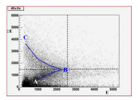
Figure 3-1: Pulse height in the  $\Delta E$  plane vs. pulse height in the E plane in ADC channels. The dotted line represents the "punch-through" point (B), while the solid line represent protons with increasing momentum from top (C) to bottom (A). This plot which includes all the counters in the E and  $\Delta E$  planes was produced after first matching the gain of the different paddles inside the E and  $\Delta E$  planes.
