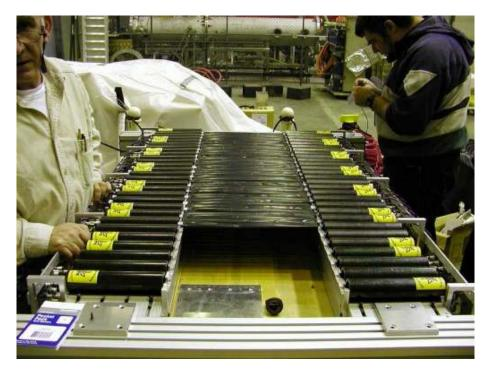
Figure 2-9: The auxiliary plane during assembly.
