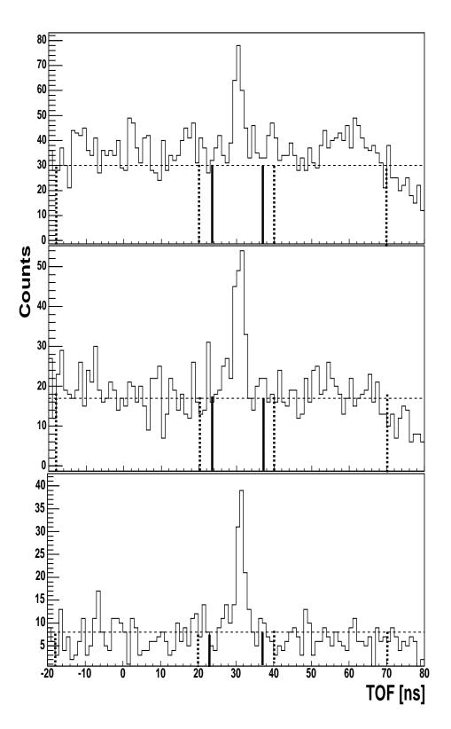
Figure 4-7: The corrected TOF between the target and BigBite E plane for K1, K2 and K3 kinematics from top to bottom respectively. The vertical lines represent the edges of the signal, while the dashed vertical lines represent the edges of the background windows.
