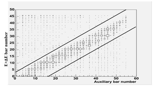
Figure 3-15: The distribution of the hit bar number in BigBite Trigger plane (E+DE) vs. the Auxiliary plane bar number. The area between the two diagonal lines was selected in order to remove neutral and negatively charged particles tracks.
