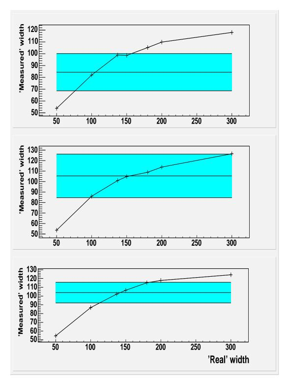
Figure 4-11: 'Measured' vs. 'real' width of the c.m. motion in the vertical direction for K1, K2 and K3 (top to bottom). The curve is a result of the simulation described in appendix B. The middle horizontal line in each plot represents the width from the data. The top and bottom lines define one standard deviation from the central value.
