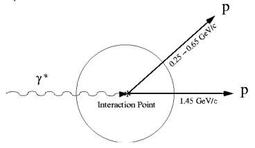
Figure C-4: The schematic of the conditioned transparency calculation for the two protons in the triple coincidence experiment.
