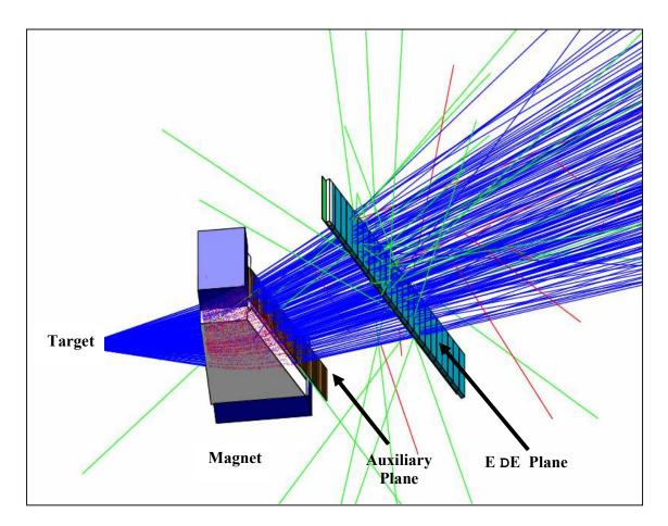
Figure B-1: A GEANT4 schematic view of BigBite with simulated 400 MeV/c proton tracks (dark) and neutrons tracks (bright).
