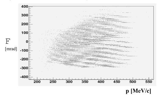
Figure 3-11: A Scatter plot of the out-of-plane vertical angle [mrad] vs the proton momentum [MeV/c] for proton singles. The angular acceptance of BigBite is limited at momenta lower then < 350 MeV/c.
