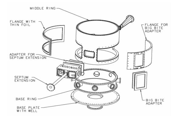
Figure 2-4: Exploded view of the scattering chamber. The septum extension was not used in this experiment.
