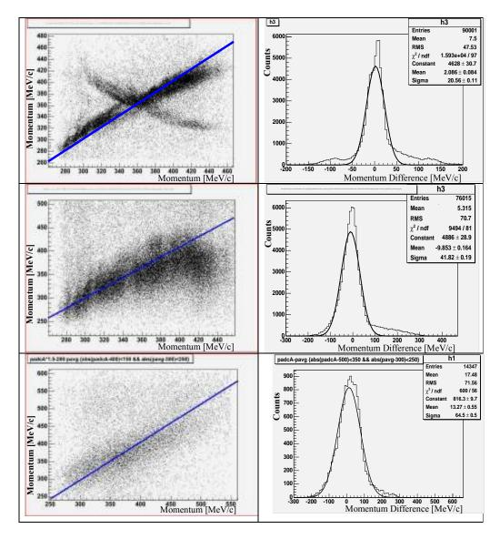
Figure 3-4: Reconstructed momentum using energy deposit vs. proton deduced from the over-determined H(e,e'p) reaction (Left). The difference of the two reconstructed momenta (Right). From top to bottom- Reconstructed momentum using energy deposit in the E plane (Top), using energy deposit in the DE plane (Middle), and using energy deposit in the auxiliary plane (Bottom).
