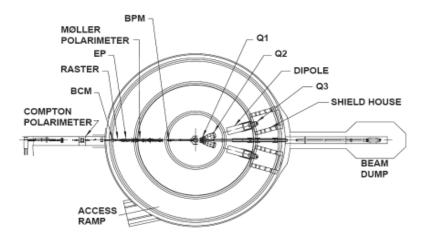
Figure 2-3. Schematic layout of Hall A, indicating the location of the raster, the ep energy measurement system, the beam current monitors (BCM) and the beam position monitors (BPM) upstream of the target. Also indicated are the locations of the components of one of the high-resolution spectrometers (Q1, Q2, dipole, Q3 and shield house) and of the beam dump. The beam polarimeters shown in this figure were not used in this experiment.
