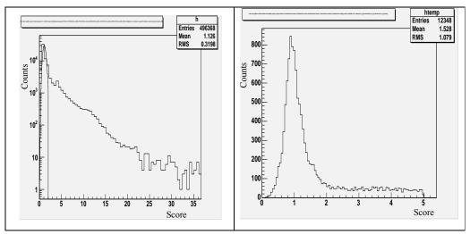
Figure 3-10: Left: The score calculated for the Elastic data events viewed on a log scale. The narrow peak represents simulated results with no accidentals. Right: a zoom in of the score distribution calculated for the elastics data events. Applying a score< 2 cut to the simulated distribution, resulted with about 1 percent event loss. A similar cut on the data removes about 30 % of the total events.
