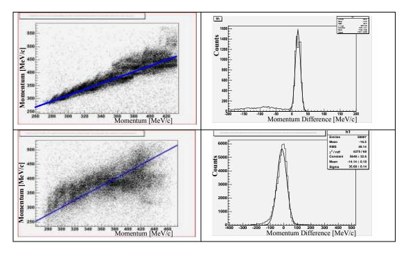
Figure 3-2: Reconstructed momentum using TOF vs proton momentum deduced from the H(e,e'p) reaction using the electron in the HRS (Left). The difference of the two reconstructed momenta (Right). Momentum reconstruction using TOF between the target and the E plane (Top). Using TOF between the Auxiliary plane and the E-plane (Bottom).
