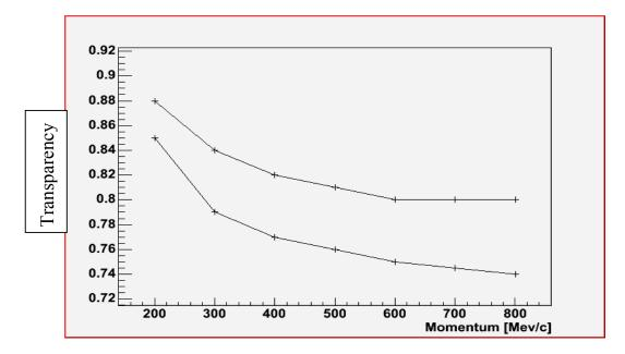
Figure C-5: The Transparency and conditioned Transparency (upper plot) as a function of the momentum of the recoil particle.
